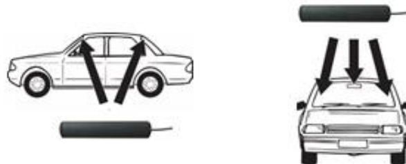
Figure 10: Sample Cellular Mounting Locations – automobile example
