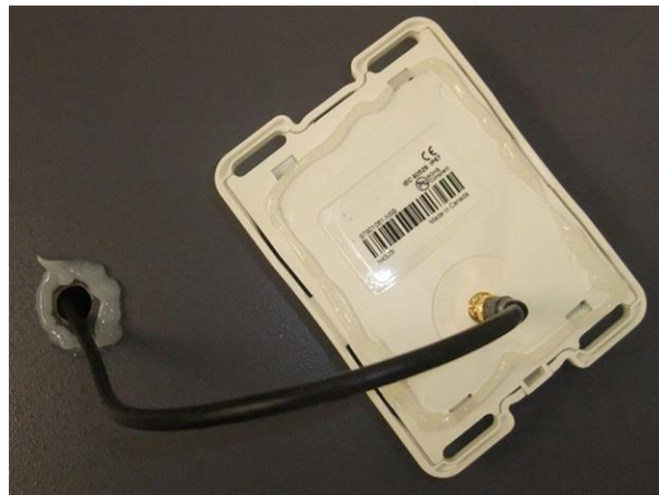
Figure 9: Apply Silicone to Hole in Asset
