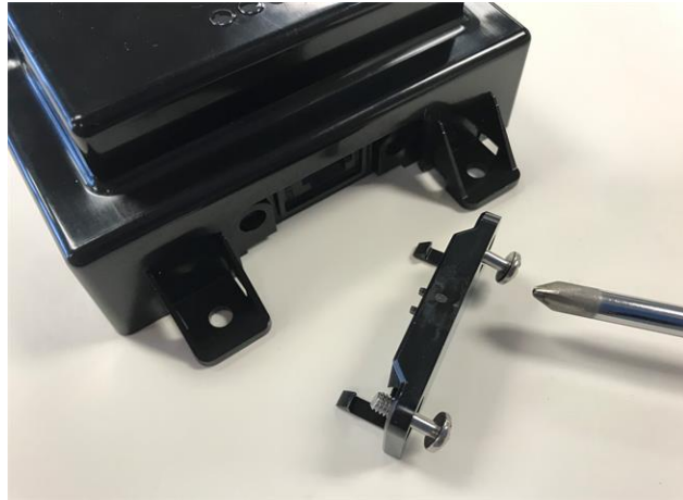
Figure 1: Remove SIM Card Door
