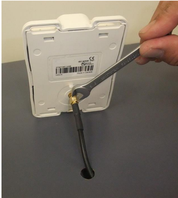
Figure 8: Attach Cable to Transceiver
