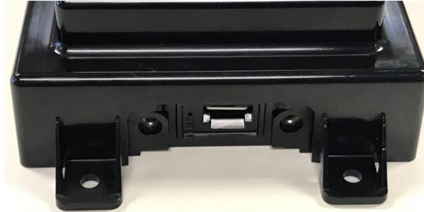
Figure 4: SIM Card Installed
