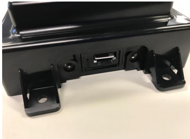
Figure 2: Remove any Existing SIM Card
