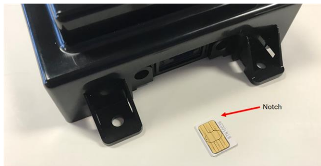
Figure 3: Sample SIM Card Orientation
